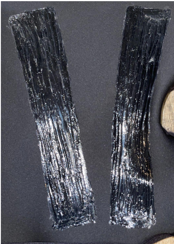
Silicone paint application on the fabric surface inside the CS prototype.
